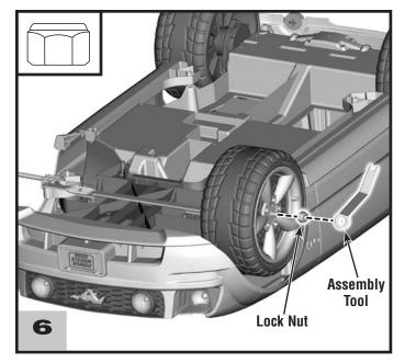
• Fit a <sup>3</sup>/8"-16 lock nut, *rounded side out*, onto the front axle. **IMPORTANT!** Tighten the lock nut **firmly** with the closed end of the assembly tool.
